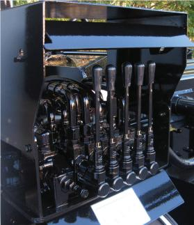
Integrated main hydraulic control valve with tarper mounting platform
