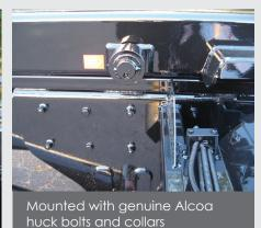
Custom fender mounts that are huck bolted to chassis frame rail
